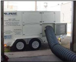
Fig. 1. Mobile Heat Treatment Unit
